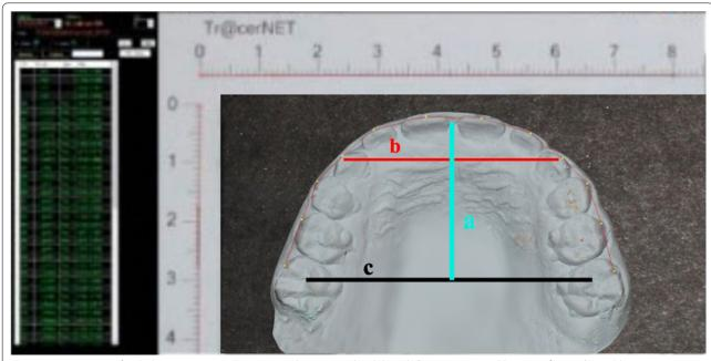
Fig. 1 Measurement of arch dimensions using TracerNet, a showing total arch length, b intercanine width, c inter-first-molar width
