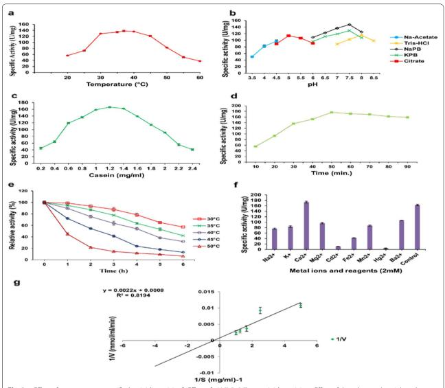
**Fig. 2** a Effect of temperature on purified actinidin activity. **b** Effect of pH (3.5–8.5) on actinidin activity. **c** Effect of the substrate (casein) on the actinidin activity. **d** Effect of incubation time on the actinidin activity. **e** Effect of temperature on actinidin stability. **f** Influence of metal ions (2 mM) on actinidin activity. **g** Lineweaver–Burk plot of purified actinidin using casein as a substrate
