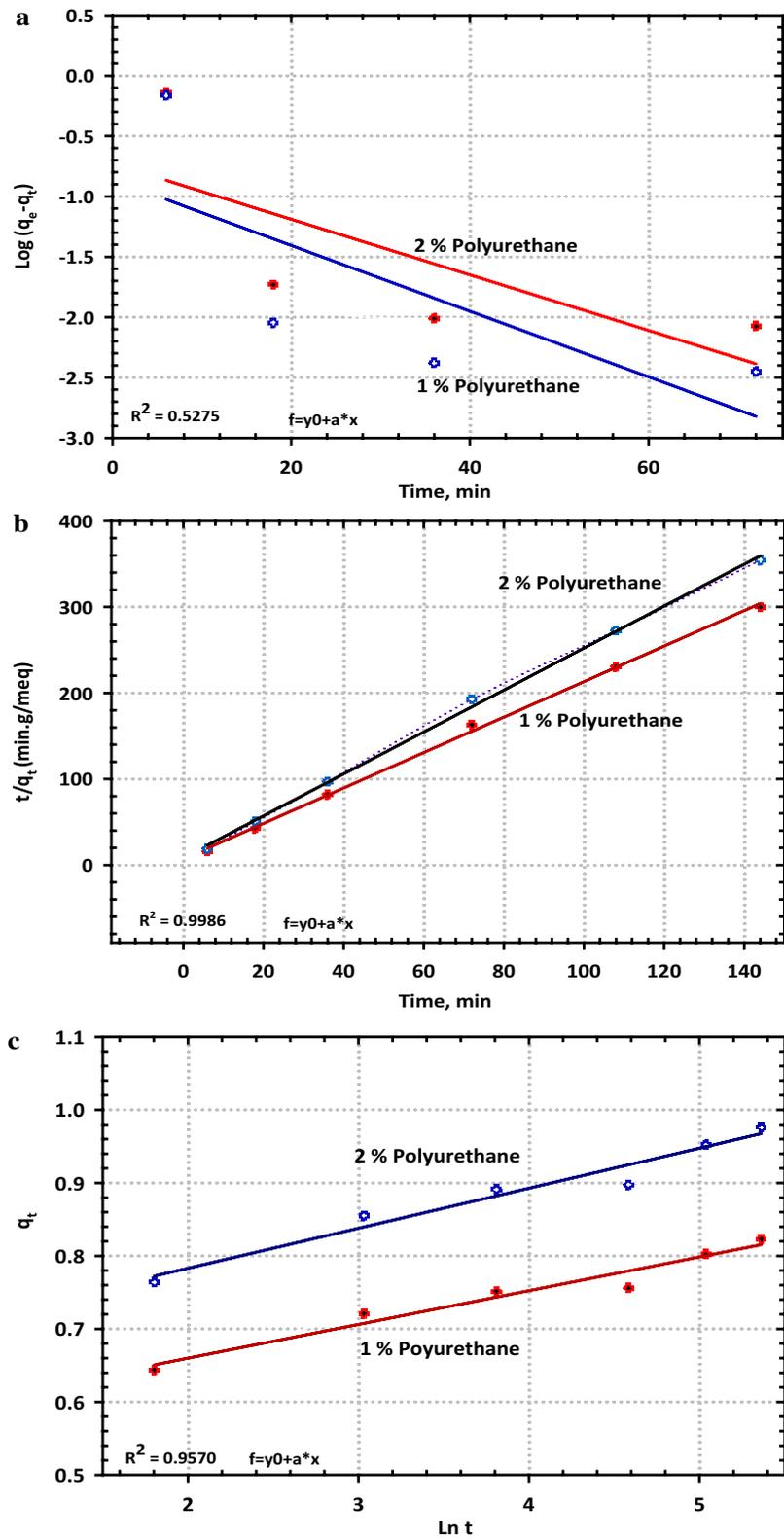
**Fig. 13** Kinetic models of polyurethane **a** pseudo-first-order, **b** pseudo-second-order and **c** Elovich kinetic model
