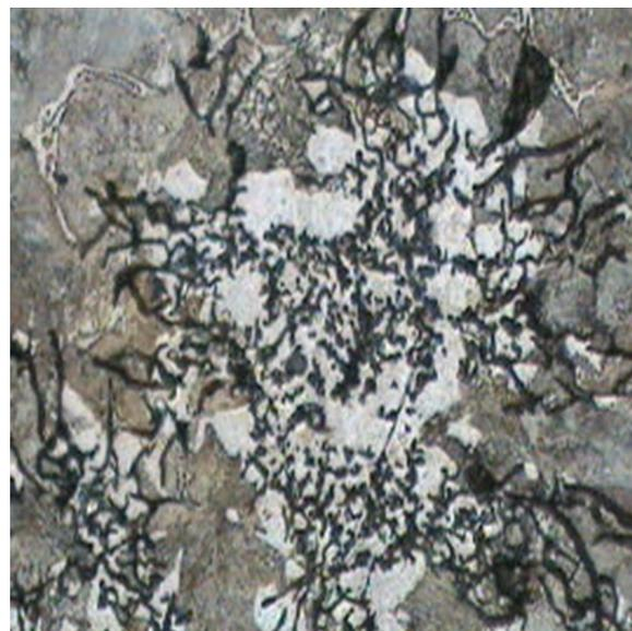
**Fig. 6** Micrograph of a metallurgical structure consisting of ferrite (light constituent), pearlite (gray constituent), and graphite flakes (dark constituent). Etched in 5% Nital,  $\times 200$
