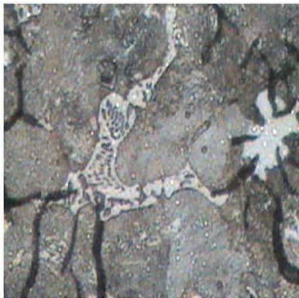
**Fig. 7** Higher magnification represents graphite flakes, cementite, pearlite, and ledeburite. Etched in 5% Nital,  $\times 500$
