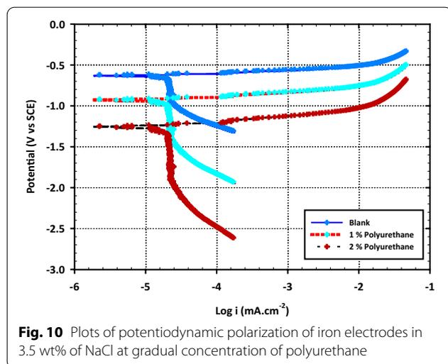
**Fig. 10** Plots of potentiodynamic polarization of iron electrodes in 3.5 wt% of NaCl at gradual concentration of polyurethane
