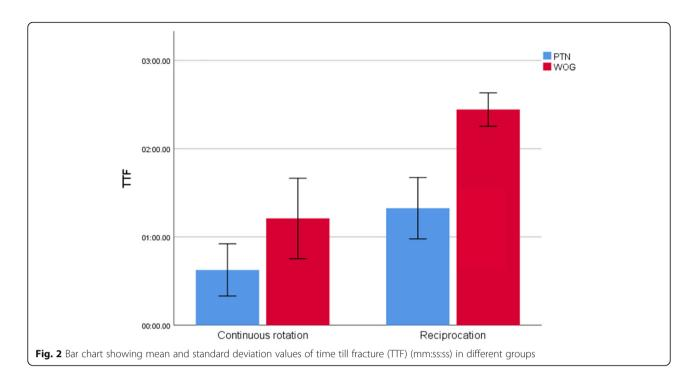
Mode. Both are pre-programmed modes, with the speed and the torque of the rotating files are not influenced by the operator. No previous study had operated the WOG in continuous rotation or the PTN in reciprocating motion. An important feature in the performance of the reciprocating instruments is the reciprocation range. The manufacturer of WaveOne rotary system suggests a range of 150 counter-clock wise/30 Clockwise that
