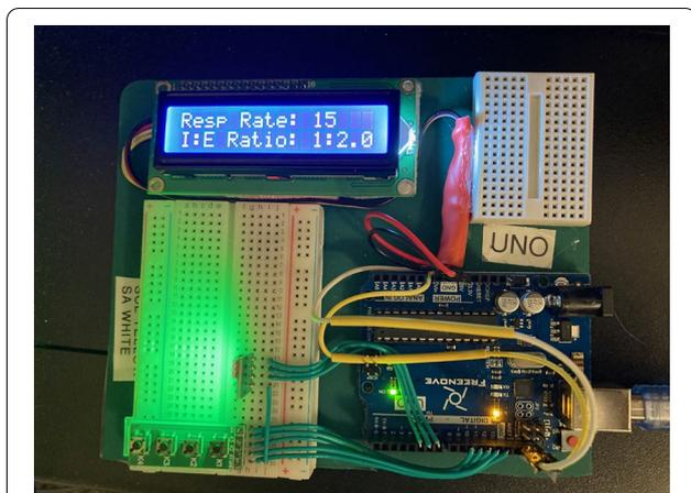
**Fig. 5** Photograph of the prototype for the advanced system corresponding to the code in Fig. 4. Note the presence of a 2-line by 16-character LCD display (for displaying the respiratory rate and I:E ratio) as well as a 4 × 1 array of pushbuttons (K1, K2, K3 and K4) used to setup (initialize) the operation of the unit. Notice also the illuminated green LED
