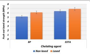
**Fig. 1** Column chart comparing total Push out bond strength mean values as impact of chelating agent group with/out laser activation
