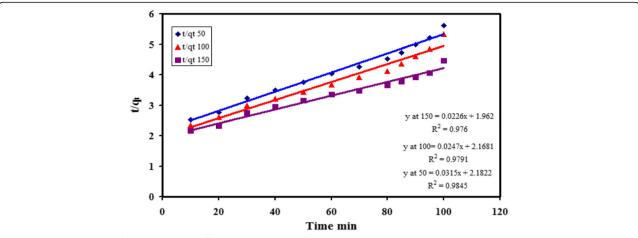
Fig. 10 Pseudo-second-order model plot at different concentration of adsorption AO67 onto RPSF [pH = 2.5, temperature 25 °C, and adsorbent dose 0.2 q]
