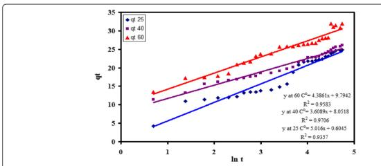
Fig. 12 Elovich equation model plot at different temperature of adsorption AO67 onto RPSF [pH = 2.5, concentration 100 mg/L, and adsorbent dose 0.2 al
