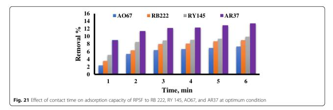
the small particle size of adsorbent the reaction is energetically favorable. The removal of different dyes (AO67, RB222, RY145, and AR37) from wastewaters may be carried out by using RPSF under optimum conditions, the effect of adsorbent more affective for dye AR37 than dyes AO67, RB222, and RY145).
