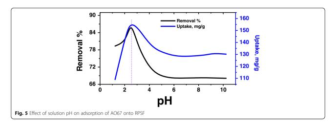
from 0.02 to 1.0 g, dye removal efficiency was increased from 75.4 to 88.5 at  $0.2 \,\mathrm{g}/40 \,\mathrm{mL}$  and then decreased to 52.6% at  $1.0 \,\mathrm{g}/40 \,\mathrm{mL}$ . This phenomenon was observed at the dye concentration studied. The increase in percentage removal with the adsorbent dose can be attributed to the increase of the available sorption surface and availability of more adsorption sites (Meena et al. 2012)
