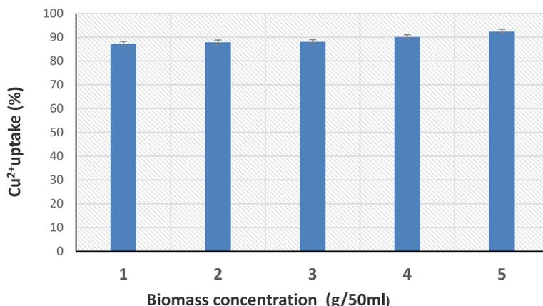
**Fig. 2** Effect of biomass concentration on Cu<sup>2+</sup> uptake by *Aspergillus tamarii* NRC 3 biomass (Cu<sup>2+</sup> conc., 80 ppm)
