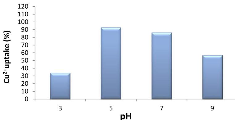
**Fig. 3** Effect of initial pH on Cu<sup>2+</sup> uptake by *Aspergillus tamarii* NRC 3 biomass (Cu<sup>2+</sup> conc., 80 ppm)
