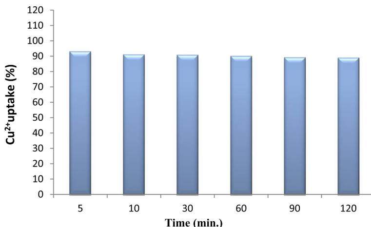
**Fig. 5** Effect of time course on Cu<sup>2+</sup> uptake by *Aspergillus tamarii* NRC 3 biomass (Cu<sup>2+</sup> conc., 80 ppm)
