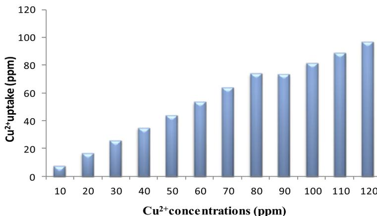
**Fig. 1** Effect of Cu<sup>2+</sup> concentration on Cu<sup>2+</sup> uptake by *Aspergillus tamarii* NRC 3 biomass (pH 5; temp, 30 °C; rpm, 150; biomass dosage, 5 g; contact-time, 1 h)
