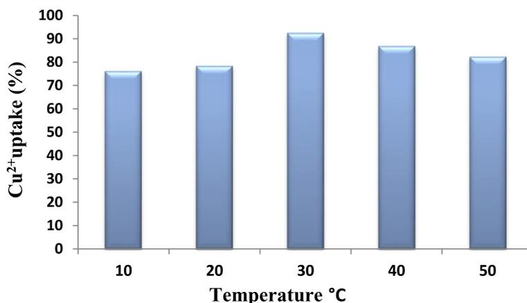
**Fig. 4** Effect of temperature °C on Cu<sup>2+</sup> uptake by *Aspergillus tamarii* NRC 3 biomass (Cu<sup>2+</sup> conc., 80 ppm)
