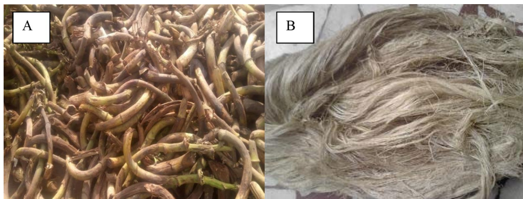
Fig. 1 A Banana peduncles. B Banana peduncle fibre after extraction (Ezeh et al. 2020)
