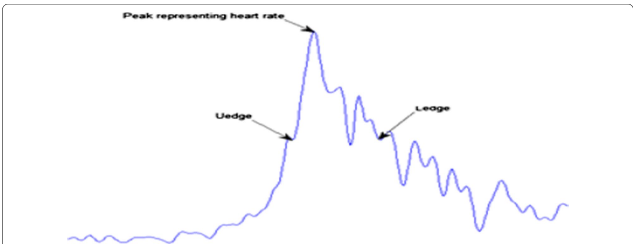
Fig. 6 Fundamental frequency and 3db points on FFT signal: Fundamental frequency in this figure represents the average heart rate of the signal where most of the information is preserved in fundamental frequency and standard 3db points have taken on either side of fundamental frequency peak to find out the wobbling of the heart rate
