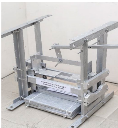
Fig. 2 Core forming machine fabricated for this study
