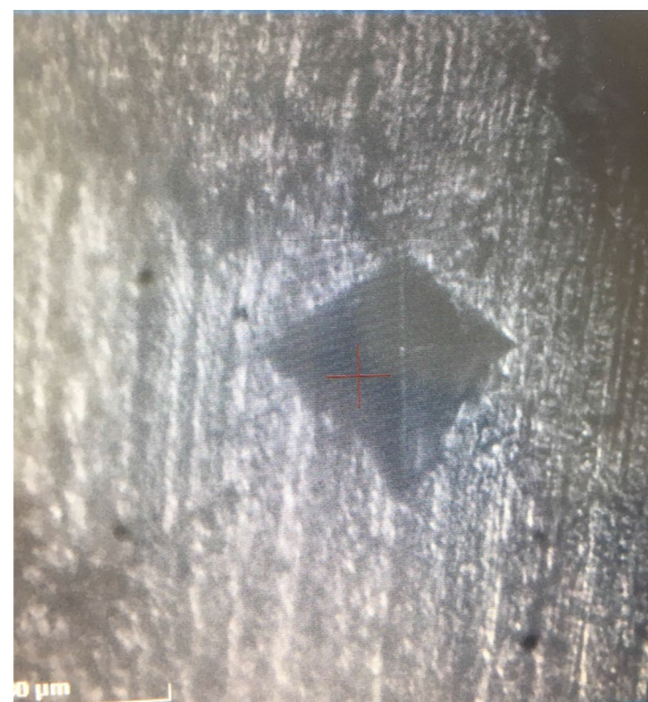
Fig. 1 A photomicrograph of Vicker's indenter on a middle section of the root after application of Moringa oleifera leaf intracanal medicament
