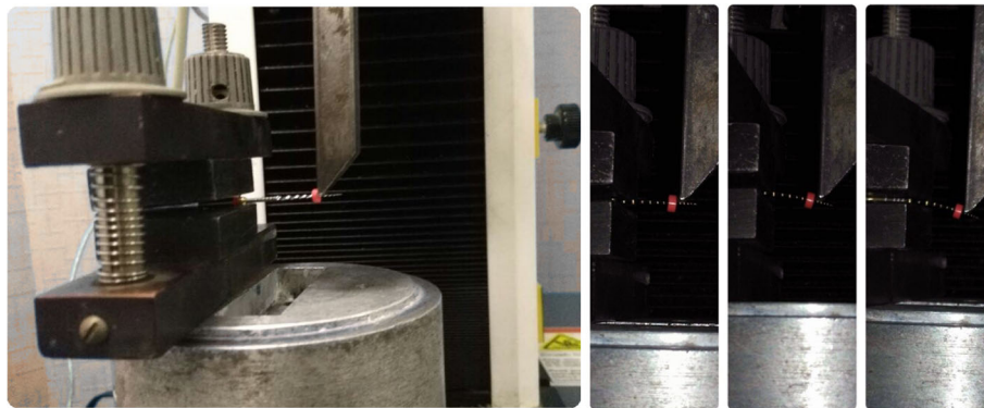
Fig. 1 Laboratory cantilever bending test of NiTi instrument
