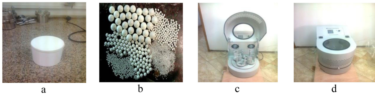
Fig. 1 PM 100 Planetary Ball-mill parts: bowl (a), balls (b), bowl's tray (c), and complete closed unit (d)
